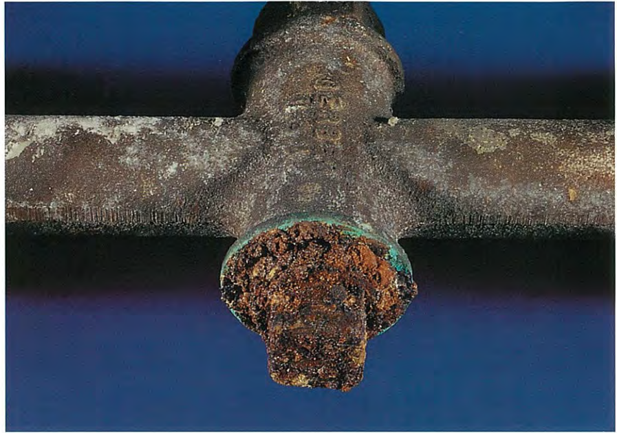
FIGURE 14 Steel nipple used to close bronze valve.
