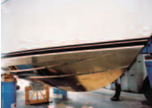
Figure 9 — Copper-nickel alloys resist corrosion and biofouling, properties exploited in hull sheathing.
