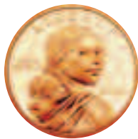
Figure 8 — Most modern coins are made from copper, copper-nickel and, in the U.S. Sacagawea dollar, a complex manganese brass. Clad and bimetallic structures add beauty and impart unique electrical/magnetic signatures that thwart counterfeiting.
