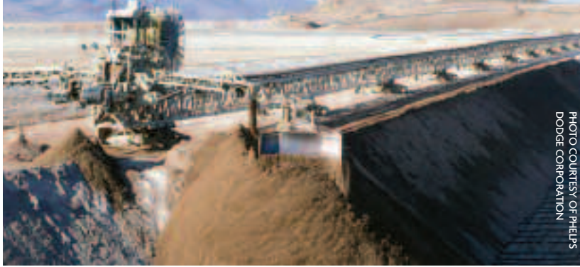
Figure 2 — Bioleaching, as shown here at Phelps Dodge's Morenci, Ariz., operations, uses natural bacteria to oxidize copper-bearing sulfide minerals, thus making it possible to apply leach/solvent extraction/electrowon to extract copper economically.
