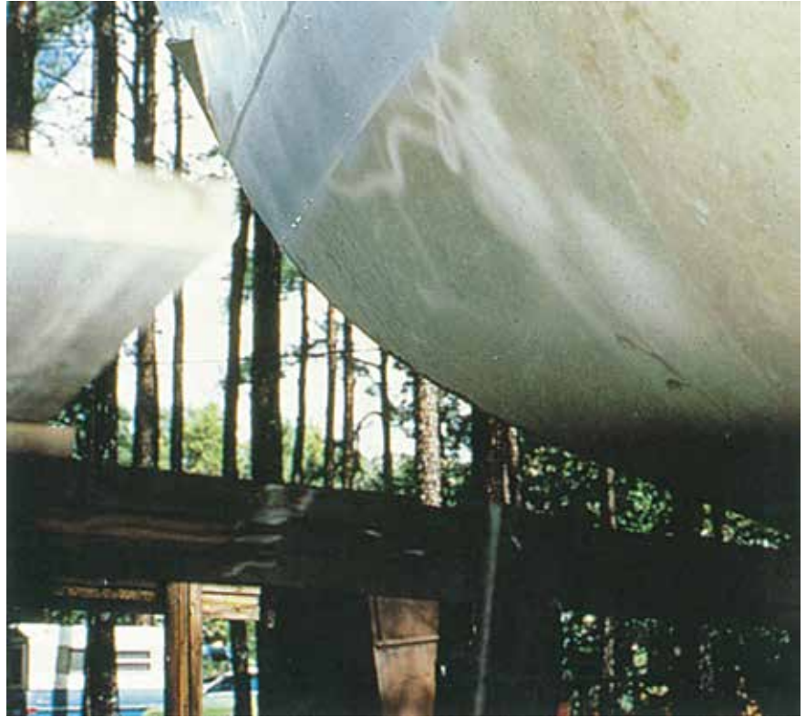
The 70-30 copper-nickel hull of the Asperida after 12 years in service
