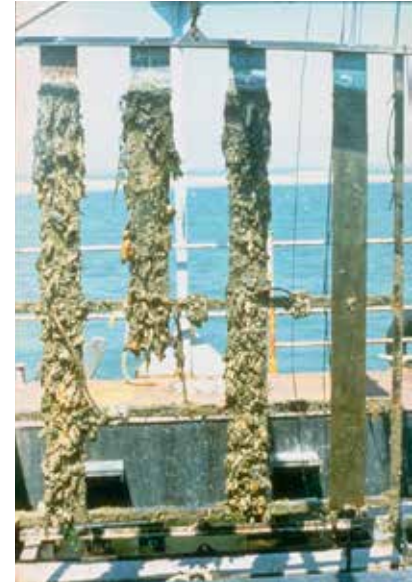
Exposure panels (left to right in above picture): steel, 90-10 copper-nickel sheathed steel, copper-nickel - all three protected with aluminium anodes - and freely exposed copper-nickel. After 12 months exposure at Langstone Harbour, UK, there was no macrofouling on the freely exposed panel
