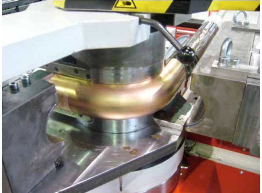
Rotary draw bending copper-nickel pipe using a mandrel (Courtesy Eucaro Buntmetall GmbH)
