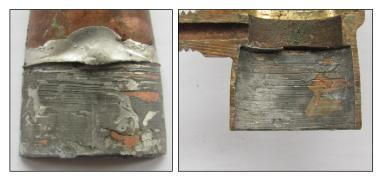
**Figure 1:** improperly Heated Solder Joint – Brush marks from mechanical cleaning (stainless steel brush inserted in power drill) still evident in soldered surface indicating inadequate heat in the tube surface leading to a lack of solder fill in the capillary space.
