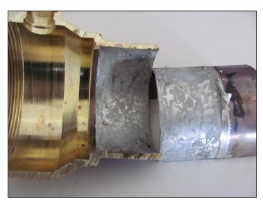
**Figure 3:** Properly Completed Solder Joint – Prepared identically to **Figure 1**. Brush marks from mechanical cleaning (stainless steel fitting brush inserted in power drill) no longer evident as proper heating allowed for complete solder flow and fill in the capillary space.
