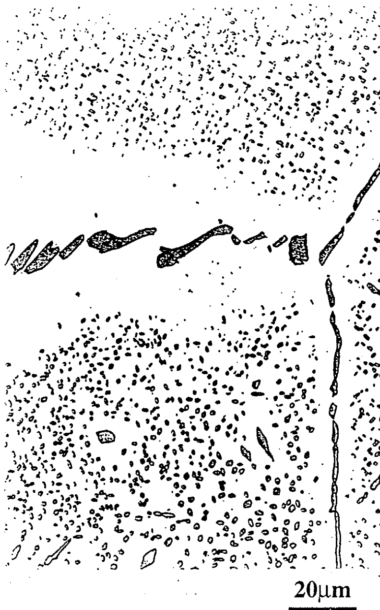
Figure 31. Light micrograph of a slowly cooled, low-aluminum NAB. No eutectoidal mixture is observed. However, there is a large number density of \kappa_{III} particles at the grain boundaries.
