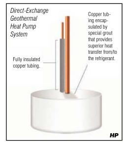
Ground-source heat pumps work by boosting below-ground temperatures, which average 50 to 60 degrees year-round, to a higher level adequate for home heating. The systems also cool homes during warm weather by returning ambient indoor heat to the ground.
