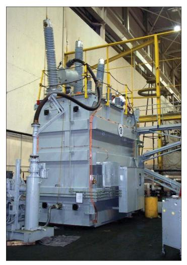
*Figure 2.* A 400-MVA, 495,000-lb transformer under construction at PTTI. The company uses copper exclusively in all its transformer product lines.
