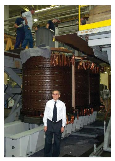
*Figure 1.* Ravi Rahangdale, president of PTTI, stands before the 90,000-lb copper coils for a 150-MVA auto transformer. Copper's high volumetric conductivity helps keep the size of what will be a 405,000-lb unit manageable.
