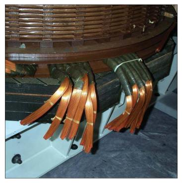
*Figure 3.* A few of many continuously transposed winding conductors in a large transformer. Copper's superior connectivity provides high reliability, an important consideration in units that typically remain in service for 40–50 years.
