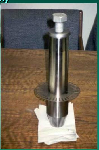
Core stack being assembled
