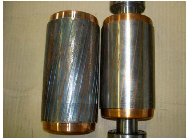
Figure 6. View of standard and higher length copper rotors, 3 kW motor.
