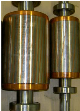
Figure 5. View of standard length copper rotors, 3 and 7.5 kW motors.
