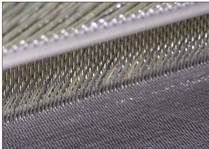
Figure 1. Dyed yarn becomes greige goods (unfinished tufted broadloom carpet) at one of Shaw Contract Division's Cartersville, Georgia, plants.
