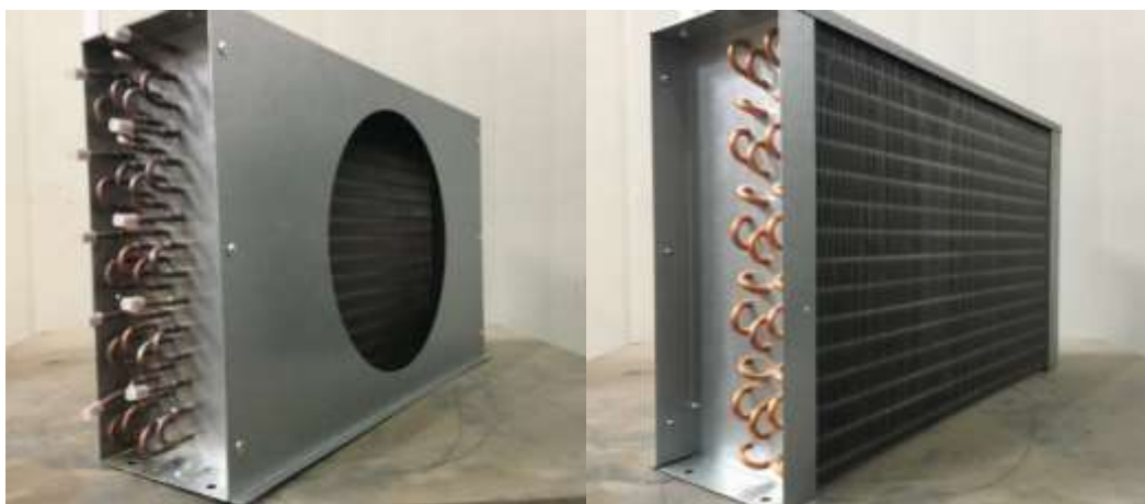
Figure 5: Photograph of C1 Prototype with sixty 5 mm copper tubes of 420 mm length in four rows.
