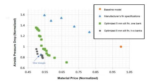
The study accomplished the objective of identifying new condenser designs that have significant potential to reduce costs and maintain performance. This is a direct demonstration of how the incorporation of smaller diameter copper tubes in heat exchange design can result in a more efficient system that reduces energy consumption and operational costs.
