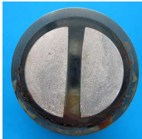
FIGURE 19: Electrode surfaces after 5 weeks under 370 Pa jet impingement at room temperature with artificial seawater containing 5 ppm hypochlorite.
