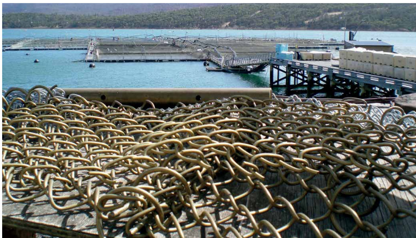
Figure 16 - Since 2005, Van Diemen Aquaculture in Tasmania has successfully used Mitsubishi-Shindoh's UR 30™ brass alloy in salmon cages supplied by Ashimori Industry Company. There are 28 salmon cages in the estuary with extreme conditions of reversing high velocity currents, salinity gradients and high summer water temperatures. (Courtesy of Van Diemen Aquaculture)
