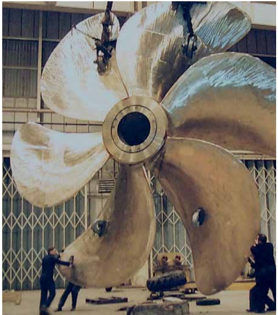
Figure 4 - Nickel aluminium bronze ship propeller (Courtesy Stone Marine Propulsion)
