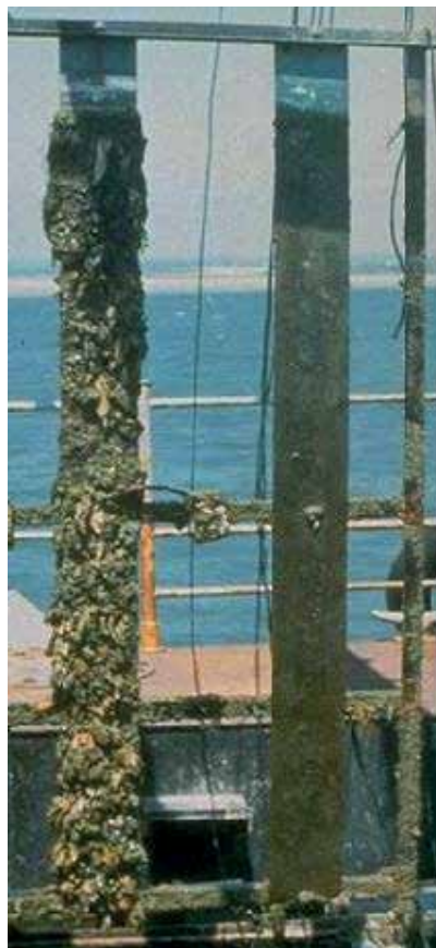
Figure 15 - Comparison of a cathodically protected (left) and freely exposed 90-10 copper-nickel panel (right) after 12 month exposure at Langstone Harbour, UK. The panel free of cathodic protection shows no macrofouling [29]
