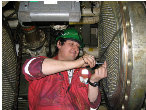
Fig 11 Eddy current inspection via a removed seawater header – there are 2,584 Cu-Ni tubes in this design
