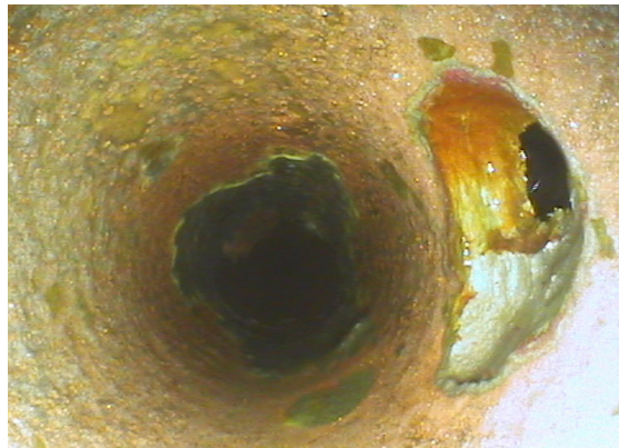
Fig 1 View along bore of failed cooler tube (7/16 inch OD) showing through wall pit
