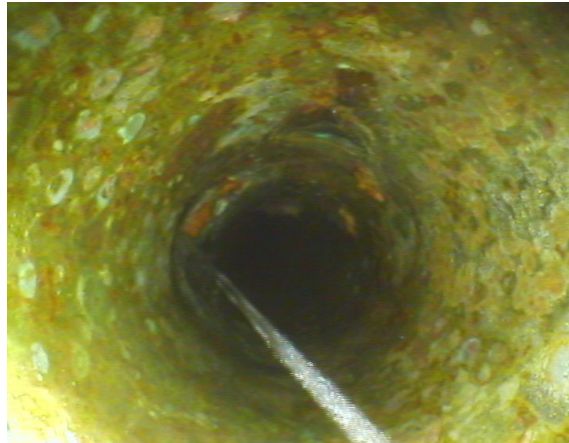
Fig 5 A pitted tube identified in a cooler using a shell side hydrostatic test and an endoscope
