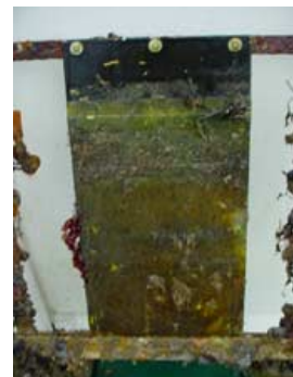
Figures 9,10 and 11. Adhesive Backed Foil panels as immersed and after 18 month and 7 year exposure
