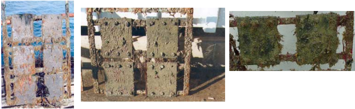
Figures 2, 3, 4. Embedded granule panels after 1, 5 and 8 years exposure
