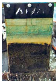
Figures 9,10 and 11. Adhesive Backed Foil panels as immersed and after 18 month and 7 year exposure
