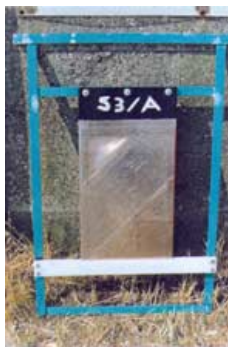
Figures 9,10 and 11. Adhesive Backed Foil panels as immersed and after 18 month and 7 year exposure
