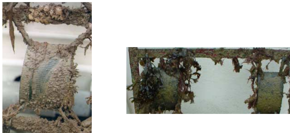
Figures 5 and 6. Expanded mesh panels after 2.5 and 7 year exposures
