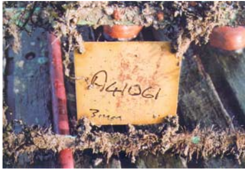
Figures 7 and 8. Hot rolled sheet after 13 month and 7 year exposures
