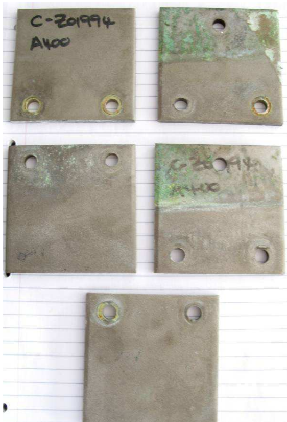
Figure 10 and 11. Nickel-copper alloy 400 samples after 6 weeks exposure; before and after cleaning
