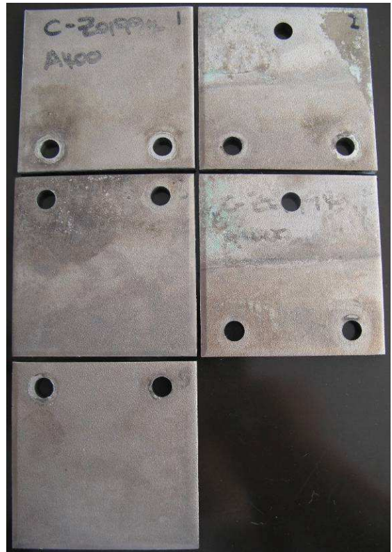
Figure 8 and 9. 70-30 copper-nickel samples after 6 weeks exposure; before and after ultrasonic cleaning.
