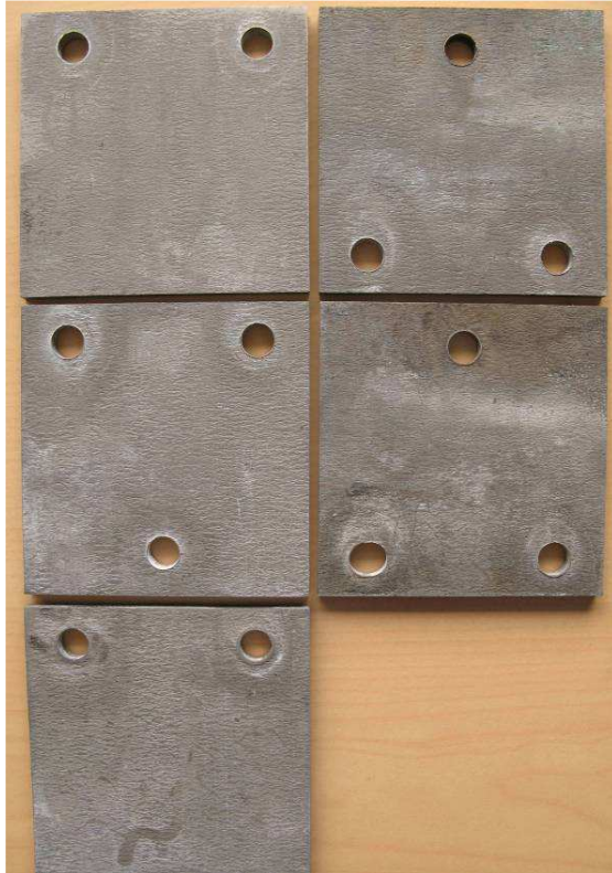
Figure 8 and 9. 70-30 copper-nickel samples after 6 weeks exposure; before and after ultrasonic cleaning.
