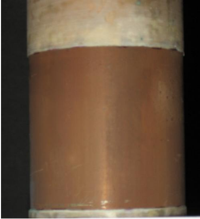
Figure 13: Surface film formed by end of 3rd trial taken several weeks after removal from the tank.
