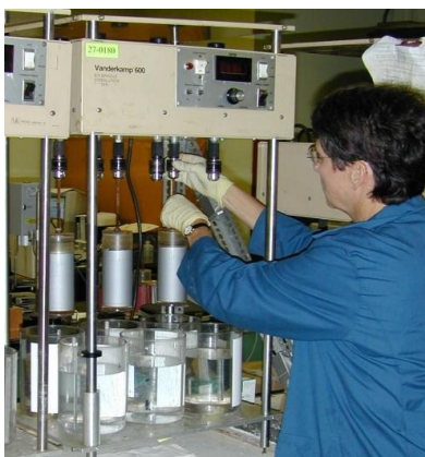
Figure 8: Attaching test cylinders to rotating apparatus.
