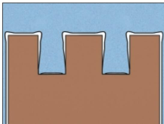
**Illustration D:** Illustration shows the uneven plating build resulting from typical mold construction practices. Chrome build up is thick on the outside corners and thin to non-existent in the channels.
