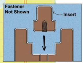
Illustration E: This illustration shows a suggested method of manufacture that results in a component that can be plated to an even thickness.
