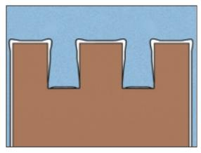
Illustration D: Illustration shows the uneven plating build resulting from typical mold construction practices. Chrome build up is thick on the outside corners and thin to non-existent in the channels.
