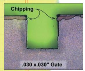
Illustration F: Chipping in gate area caused by improper removal of chrome build up at the corners.
