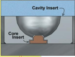
Illustration A: Use of copper alloy in cavity for thermal conductivity and plated to isolate it from the steel cavity. mal conductivity properties to improve part quality and reduce cycle times, are no different than tool steels when protection is desired.
