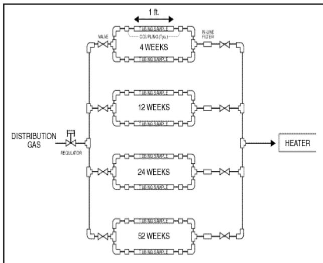
Figure 11 – Test-rack assembly
