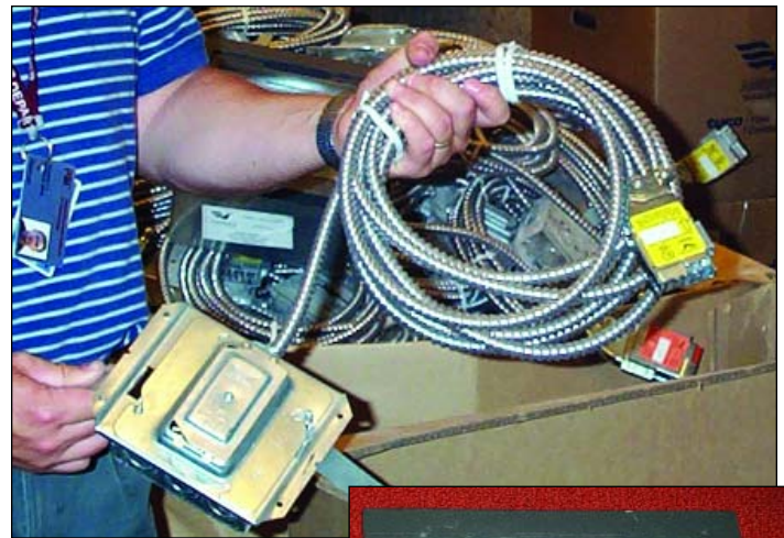
Figure 4. Modular “plug and play” outlets supplied by America Cable Systems, an AFC Company. Top: module with attached cable and connector. Bottom: outlets installed in raised flooring. Electrical specifications call for a maximum of six outlets per branch circuit, a recommended practice intended to reduce the effects of harmonics on sensitive circuits. All branch circuits also have full-sized ground wires. Cable armor, conduit and raceways are grounded but are not used in place of the primary grounding conductor.
