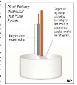
Ground-source heat pumps work by boosting below-ground temperatures, which average 50 to 60 degrees year-round, to a higher level adequate for home heating. The systems also cool homes during warm weather by returning ambient indoor heat to the ground.
