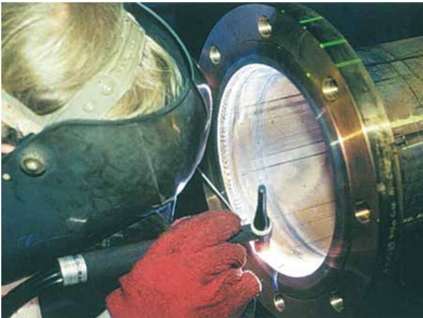
TIG (GTAW) welding a 90-10 copper-nickel assembly
