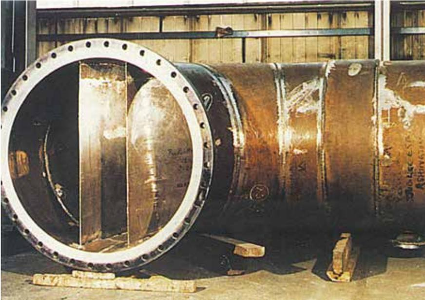
90-10 copper-nickel brine piping for a desalination plant
