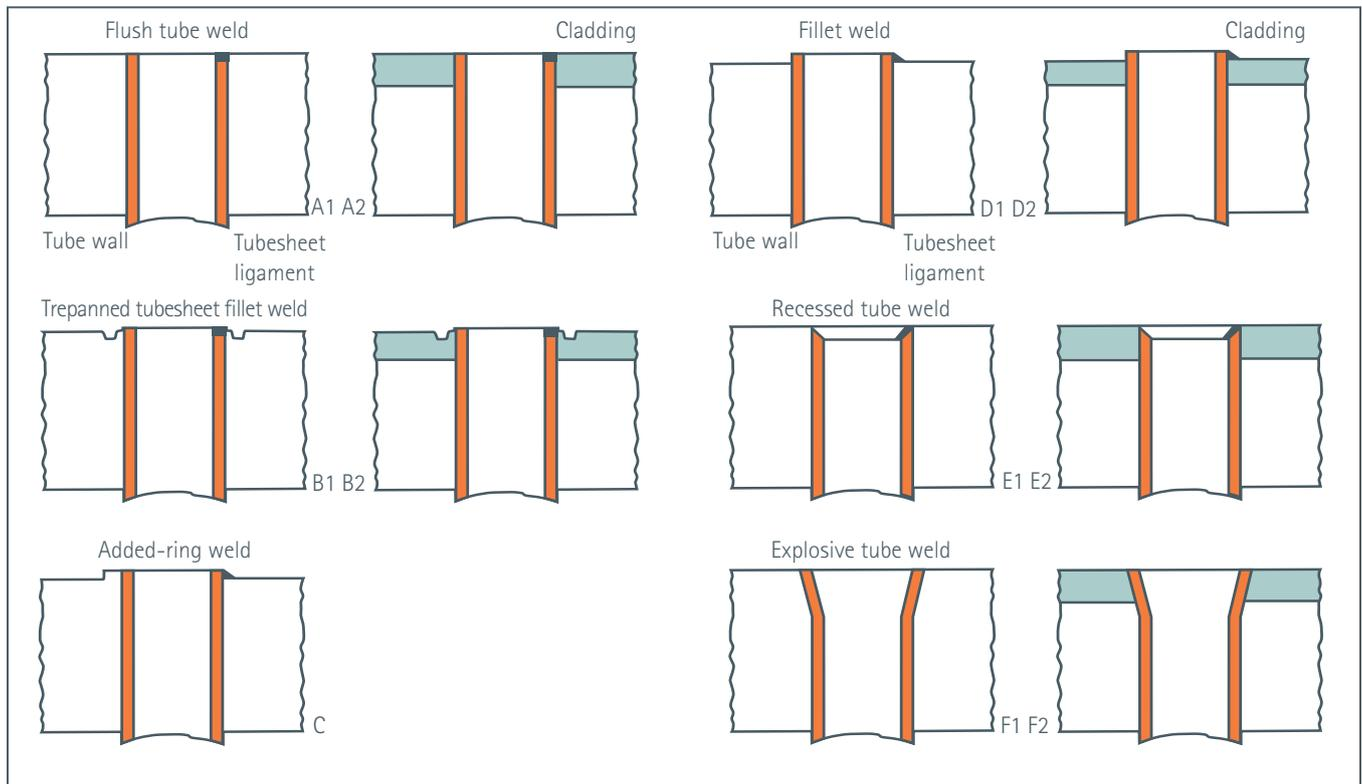
Figure 3 – Typical tube weld joint preparations showing finished weld on the right side. 1<sup>st</sup> and 3<sup>rd</sup> columns are solid copper-nickel tubesheet; the 2<sup>nd</sup> and 4<sup>th</sup> columns are clad plate (ex Reynolds et al - see Bibliography)
