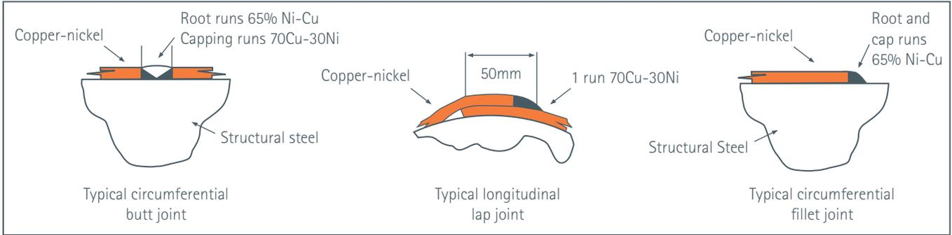
Figure 4 – Typical attachments for platform sheathing
