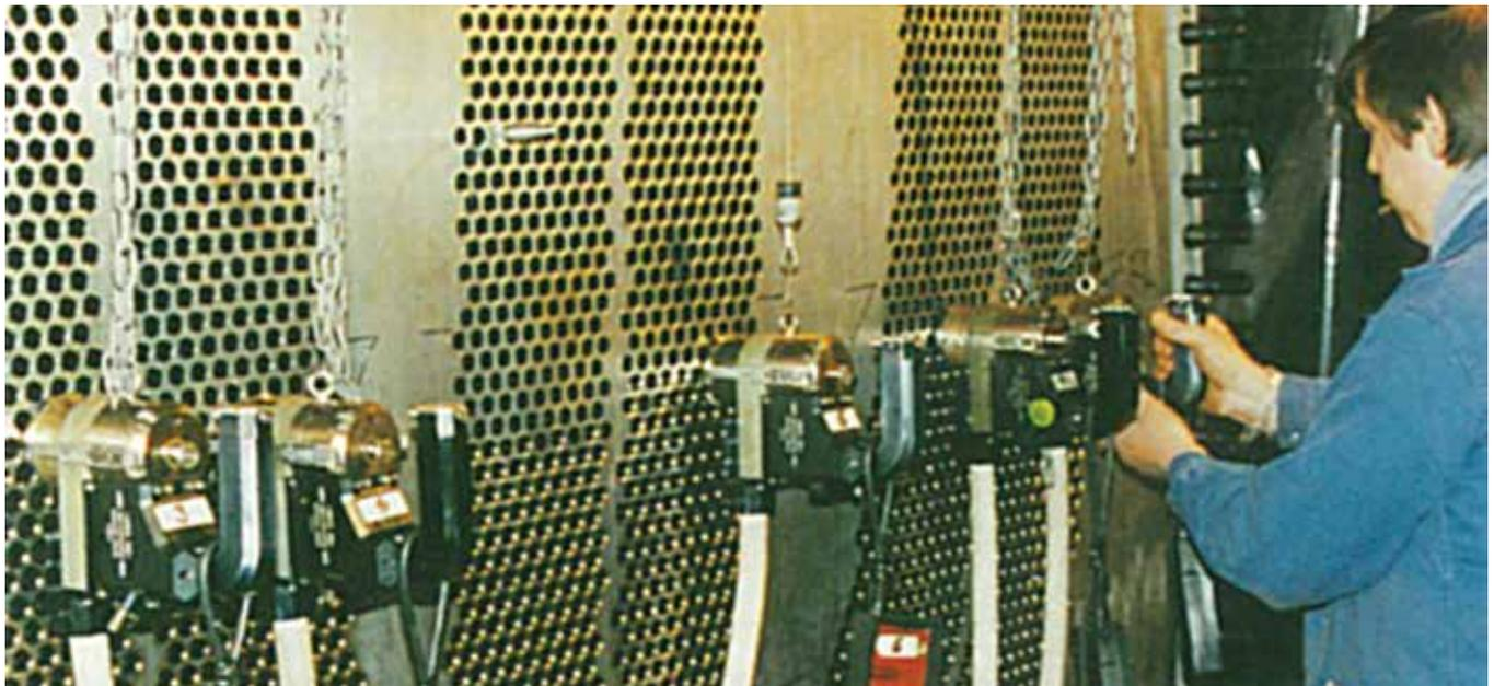
Tube to tubesheet welding of a large heat exchanger using automatic TIG (GTAW) welding heads (Courtesy Arc Machines Inc)
