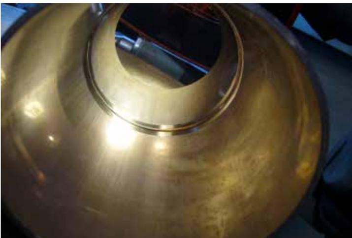
Finished weld showing root penetration on pipe bore
