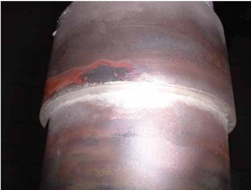
Capillary brazing of a sleeve to a pipe using a silver solder
