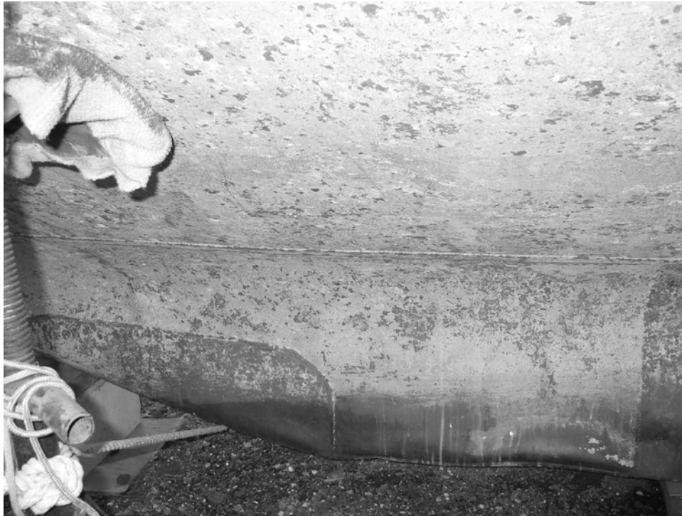
FIGURE 7: Portion of hull, portside, showing patina, horizontal lap weld and forward end of dented keel
