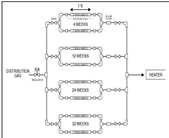
Figure 11 – Test-rack assembly
