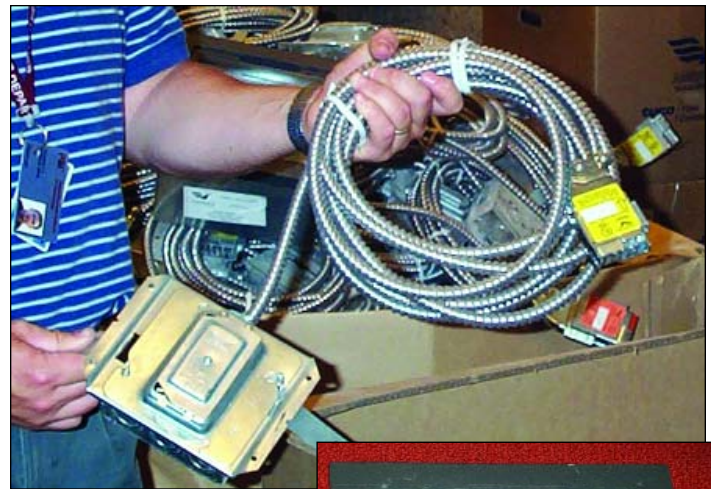
Figure 4. Modular “plug and play” outlets supplied by America Cable Systems, an AFC Company. Top: module with attached cable and connector. Bottom: outlets installed in raised flooring. Electrical specifications call for a maximum of six outlets per branch circuit, a recommended practice intended to reduce the effects of harmonics on sensitive circuits. All branch circuits also have full-sized ground wires. Cable armor, conduit and raceways are grounded but are not used in place of the primary grounding conductor.
