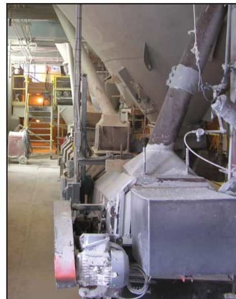
Figure 3. A 2-hp SE&A IEEE Plus belt conveyor motor (lower right of photo) that transports finely-ground product to the beneficiation department. It was one of the first copper-rotor motors installed during the current replacement program. The data plate lists the motor's NEMA nominal efficiency at 87.5%, one full percentage point higher than called for under NEMA Premium standards.
