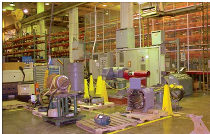
Figure 2. Kodak Park operates several large shops that cost-effectively rebuild more than 500 motors annually, many of them DC vehicle motors or special-purpose motors for which no EAct or NEMA Premium standards exist. But Kodak found that for general-purpose motors that are covered by high-efficiency standards, maximum savings are often gained by simply replacing the motors with NEMA Premium-efficiency units.
